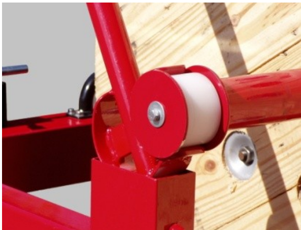
Pos. 9-10: Insert the levers into the spacers, find the pin and push downwards.
