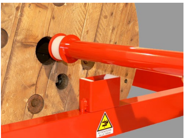
Pos. 5-6: Insert and align the rotation pin
